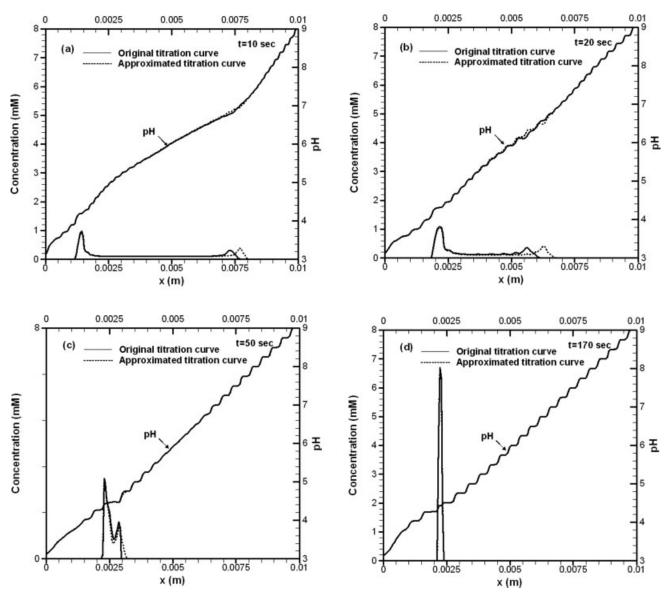
Figure 8. Comparison of pH curves and protein shape for original and approximated titration curves.
