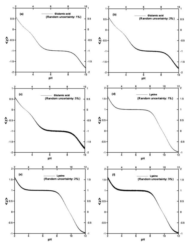
Figure 2. Titration curves with 1%, 2% and 3% random noises for glutamic acid (a, b, and c), and lysine (d, e, and f), respectively.
