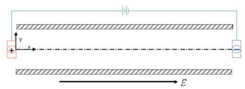
Figure 6. 2-D planar microchannel (1 cm  $\times$  100  $\mu$ m) used to simulate the ampholyte based isoelectric focusing in a pH range of 3 to 9.
