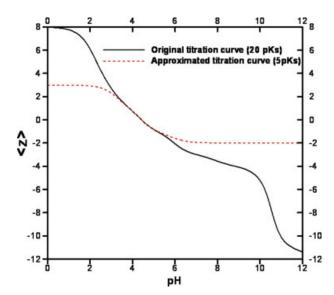
Figure 5. Comparison between the original (20 pKs) and approximated (5 pKs) titration curves.
