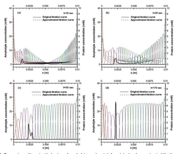
Figure 7. Comparison of transient behaviors of ampholytes and protein for original and approximated titration curves.
